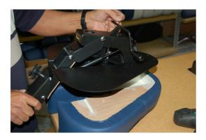
6. Place the cover on the mechanism and tighten the sctrews.
