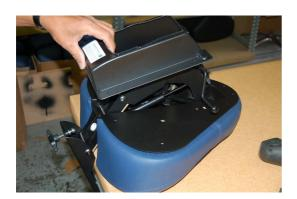
3. Unscrew the screws, holding the seat.
